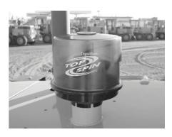
Donaldson TopSpin™ mounted on a grader. The aerodynamically designed TopSpin™ is made of a lightweight, durable, non-corroding material which makes it tolerant to all weather and operating conditions.
